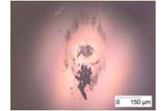
Ball surface after test
